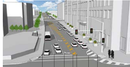
RETAIL BOULEVARD Through Lane - 3' Through Lane - 11' Left Turn - 11' Through Lane - 9' Parking Lane - 9'
